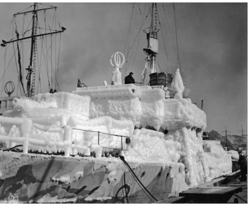
This ice-coated corvette not only shows the uncomfortable conditions at sea but also identifies the danger of sailing in winter conditions. The added top-weight of the ice affected the ship's stability and had to be removed to prevent capsizing. *DHH 81/520/1000, BOX 142 FILE 4*
